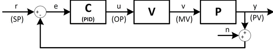
Figure 1: Feedback control loop (SISO type).
