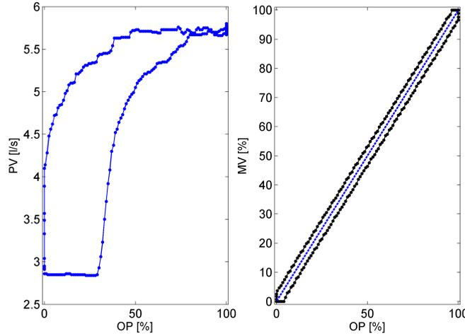
(c) Limit cycles: left) PV(OP) diagram; right) MV(OP) diagram.
