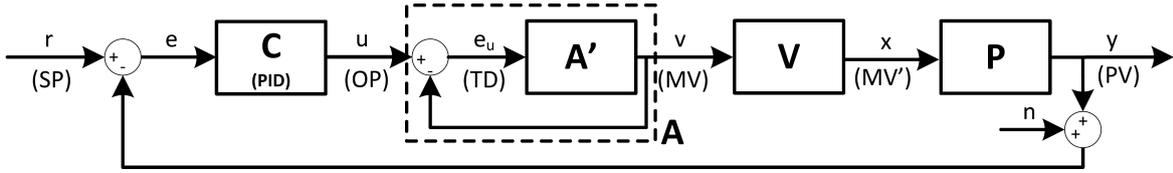
Figure 6: Control loop with “smart” electric actuator.
