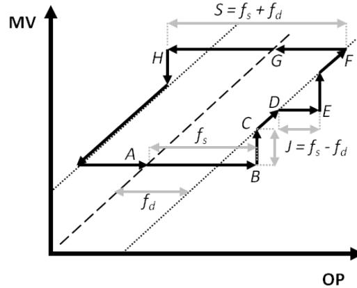
Figure 3: Modeling valve static friction (stiction). Limit cycle on MV(OP) diagram.
