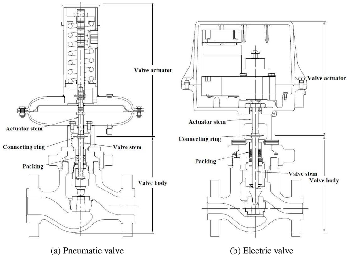
Figure 4: Example of configuration of the two different types of actuators installed on the same linear control valve.
