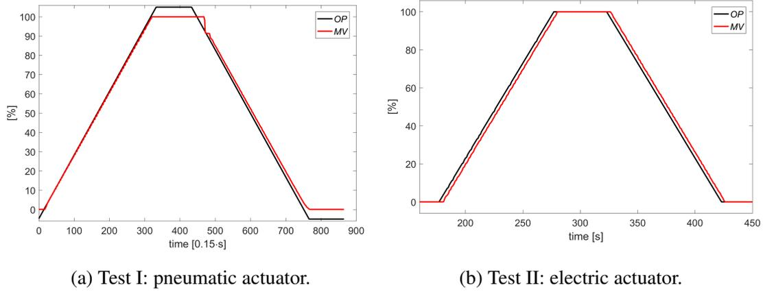
Figure 11: Time trends for tests in open-loop mode.
