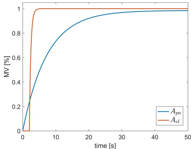
Figure 17: Comparison of step-test response for the identified dynamics of two actuators.
