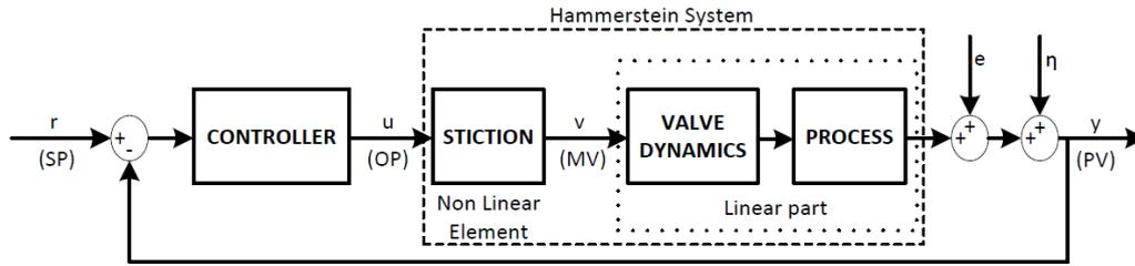
Figure 2: Hammerstein system: control valve (in friction) followed by the linear process within the control loop.
