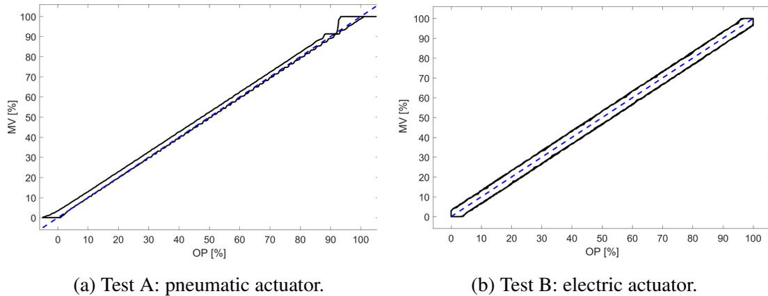
Figure 12: MV(OP) diagram for tests in open-loop mode.
