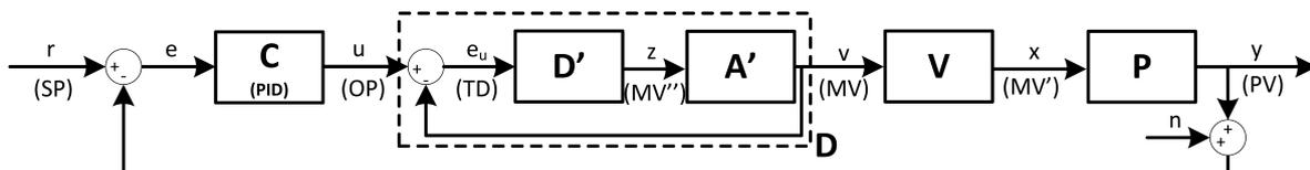
Figure 9: Control loop with “smart” electric actuator and *dead-band*.
